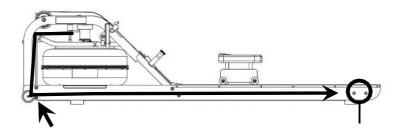
**Hint:** Before reattaching the Inner Clip/Bungee Hook, tie a slip knot under slight tension at the lower bungee pulley. This will keep the bungee under tension while reassembling the Bungee Hook.
