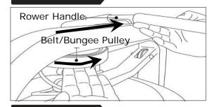
Wind the Rower Belt onto the Belt/Bungee Pulley until the Rower Handle is as it's furthest forward position.
