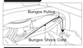
Rethread the Bungee Shock Cord (on opposite side of the Idle Wheel) back through the Bungee Pulleys and tie off at the Attachment Point.
