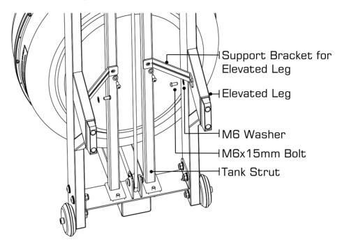
Using 4x M6x15mm Bolt[12], 4x M6 washer[8], attach the 2x Support Bracket for Elevated Leg[16] to the Rear Brace and Elevated Leg.
