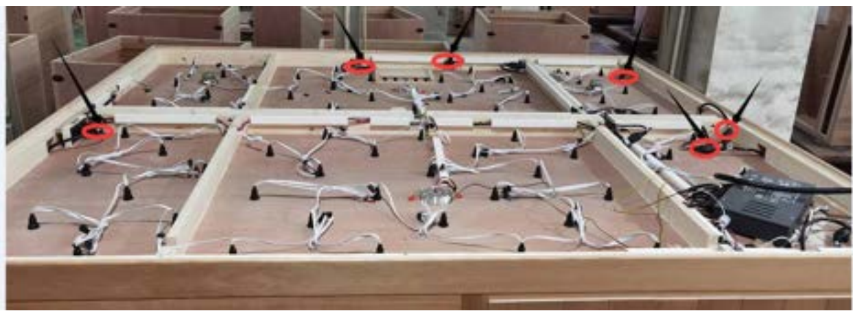
Figure 19 Connect All (6) Of The Heater Cord Connections
